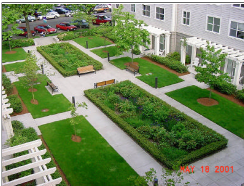
Bioretention Basin Example Source: LID Center
