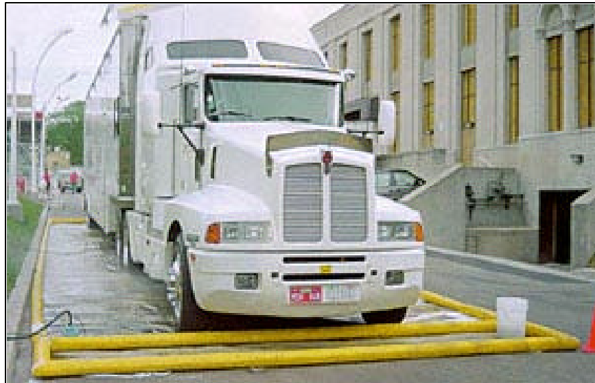
Example of a vehicle washing containment pad Source: Chappell Supply and Equipment PERMISSION PENDING
